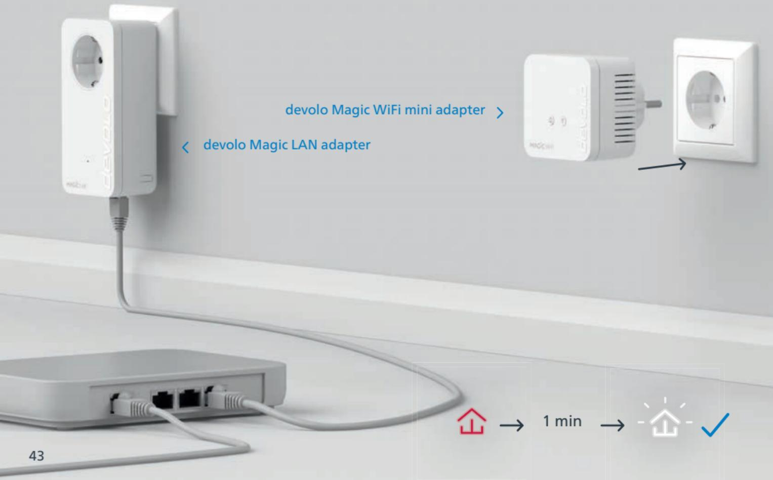
**| EN | Help: If automatic pairing during initial installation was unsuccessful, you can carry out manual pairing of the Magic adapters.** Connect the devolo Magic WiFi mini adapter to a free wall socket and wait until the LED flashes white (approx. 1 minute).
