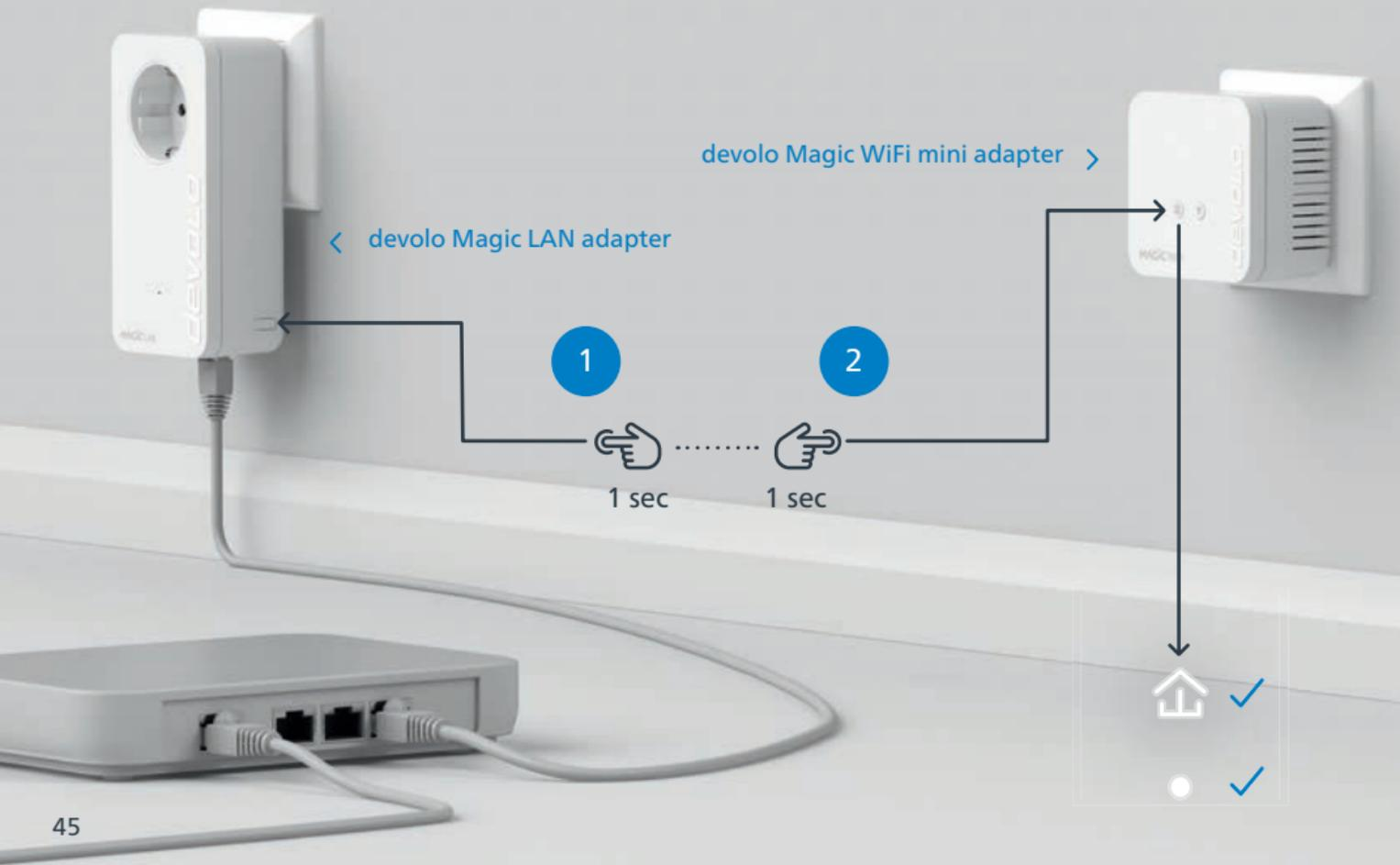
**| EN** | Within 3 minutes, press the button on the side of your devolo Magic LAN adapter which is connected to the router. Press the
