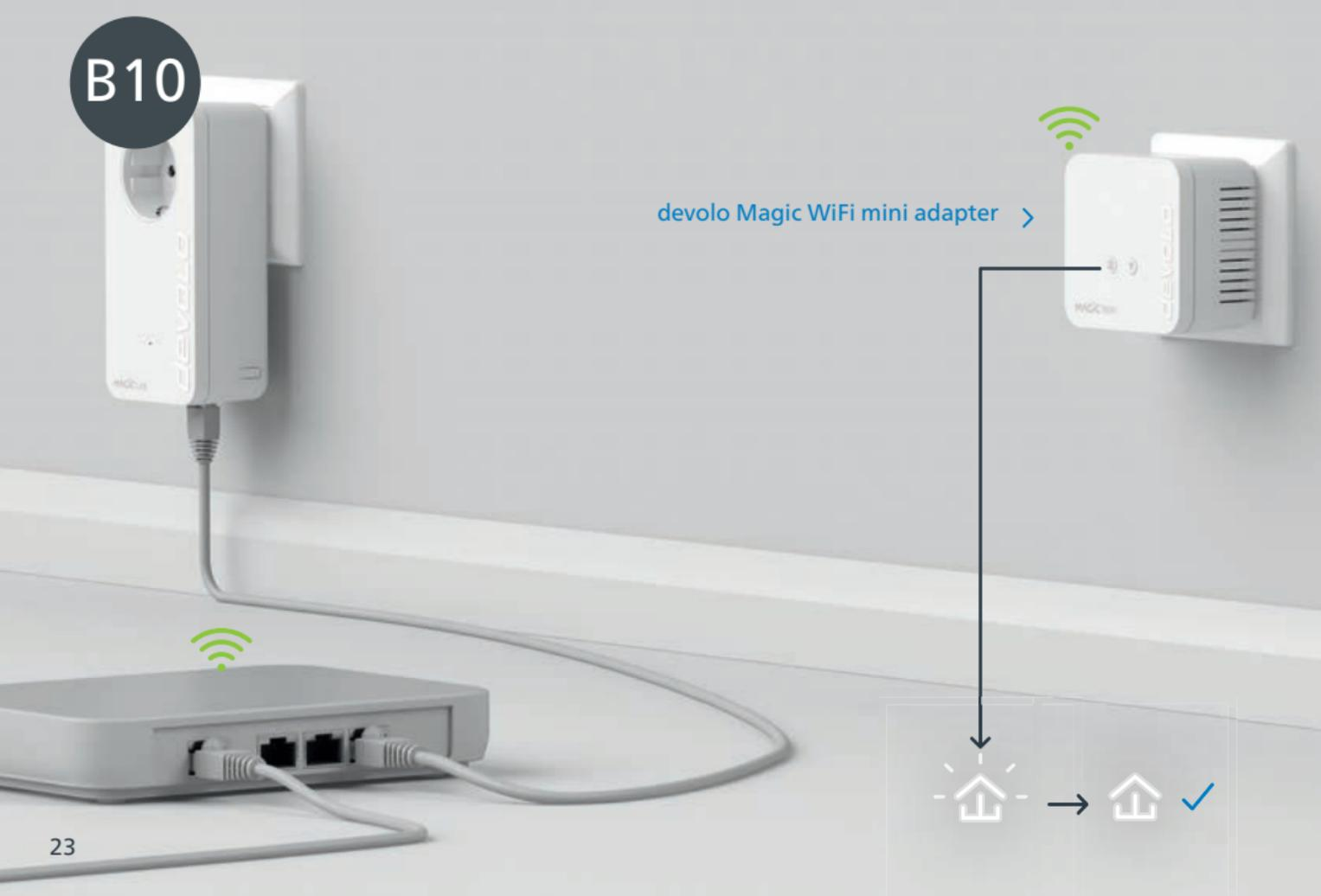
**| EN |** Once the 🏠 LED lights up solid white, the process has been completed successfully.
