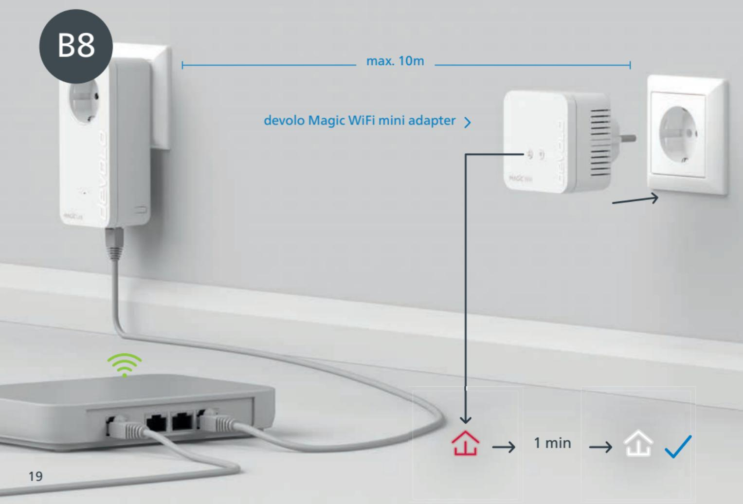
**EN** | Connect the devolo Magic WiFi mini adapter for the transmission of the Wi-Fi access data to a free wall socket near your router (max. distance 10 metres) and wait around 1 minute until the
